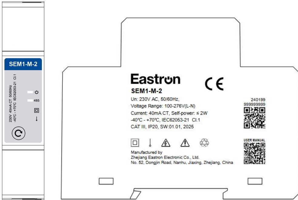
(SEM1-M-2 nameplate and laser printing)
