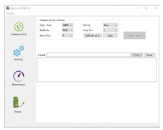
Step 3: Open the relevant terminal of the USB and set the correct parameters of the communication. The default of the meter SDM630-EV:
