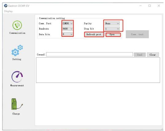
Step 4: After opening the Comm port, please click "Comm. Test" to test the communication. If the testing is OK, you will see a pop up window to show "Test succeed".
