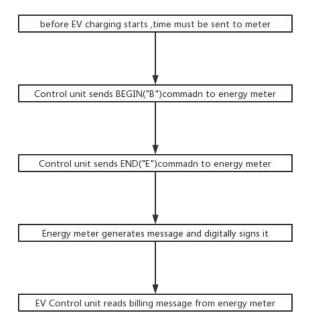
EV charger control unit must use following procedure to measure charging consumption and sign Data packet:
