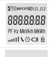
The first screen lights up all display segments and can be used as a display check.
