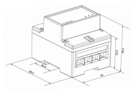
Height: 96.5mm Width: 76mm Depth: 76.5mm
