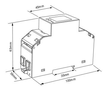
Height: 100mm Width: 36mm Depth: 63mm
