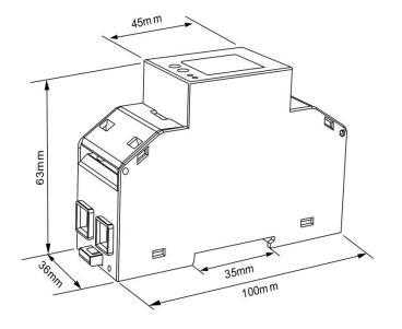
Height: 100mm Width: 36mm Depth: 63mm
