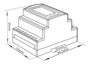
Height: 94.5 mm Width: 72mm Depth: 65mm
