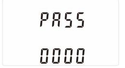
Setting up is password-protected so you must enter the correct password (default '1000') before processing. If an incorrect password is entered, the display will show: PASS Err
