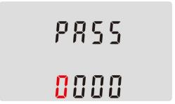
Setting up is password-protected so you must enter the correct password (default '1000') before processing. If an incorrect password is entered, the display will show: Err
