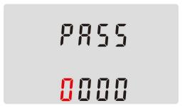
Setting up is password-protected so you must enter the correct password (default '1000') before operating. If an incorrect password is entered, the display will show: Err
