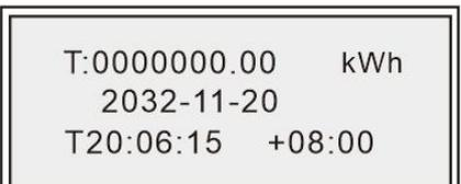
T:0000000.00 kWh<br>2032-11-20<br>T20:06:15 +08:00    | After a short delay, the screen will display active energy measurements, date, time, time zone. |
