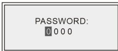
Setting up is password-protected so you must enter the correct password (default '1000') before processing. If an incorrect password is entered, the display will show: Error!
