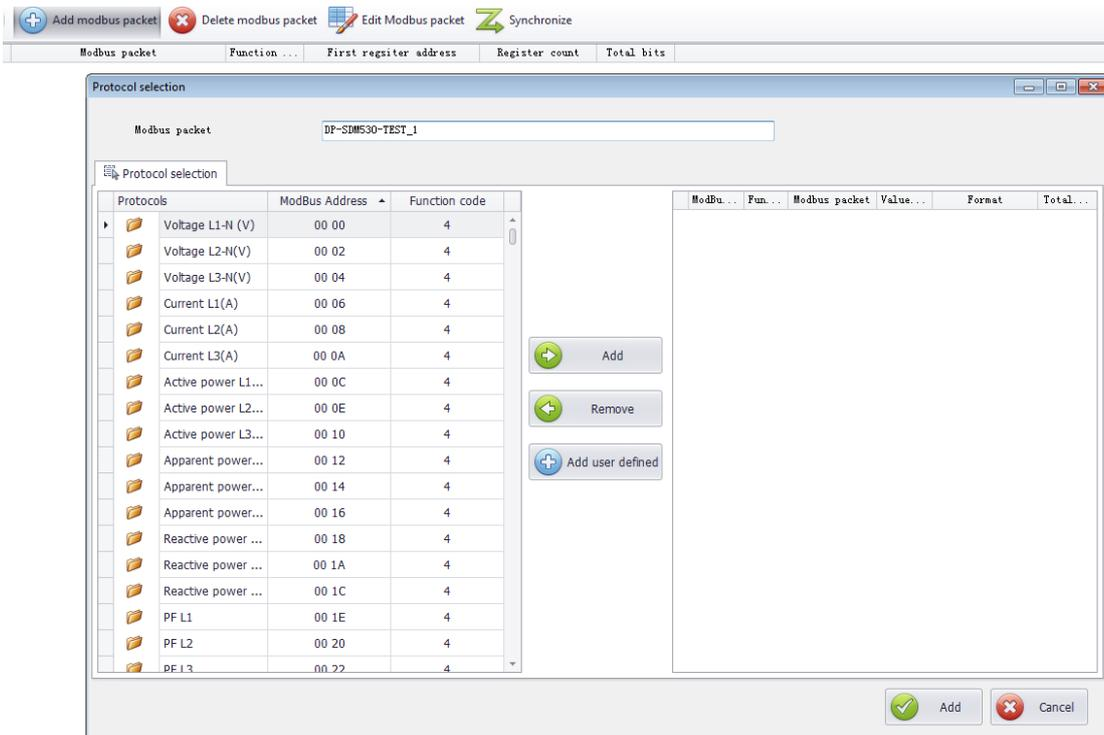
Modbus packet: means the name of the group of protocol packet, the system will have a name automatically. You can define it by your own. Normally we will use the name which system give us as default.
