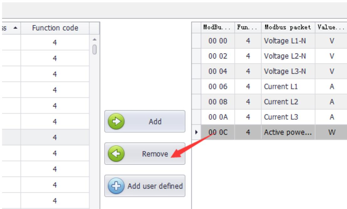
PS: When moving the protocols, only can remove them one by one. And only can remove the protocol on the head or bottom for the consistency of protocol.
