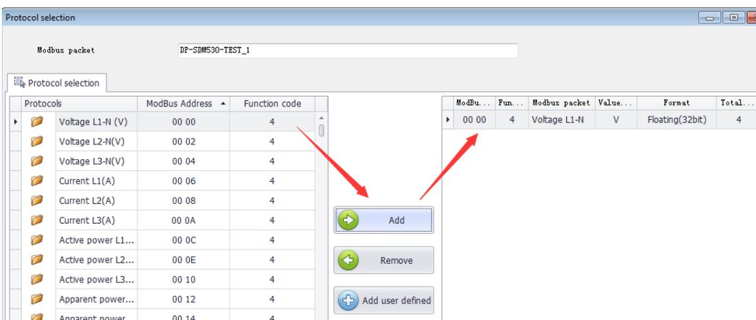
Many continuous protocols can be adding. Discontinuous protocols can't be adding.
