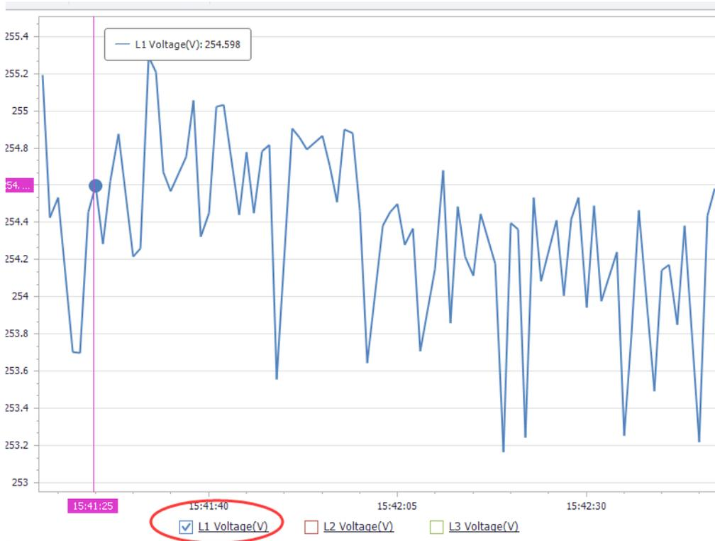
Move the cursor to left or right on the curves, the software will show the real-time reading Vernier.
