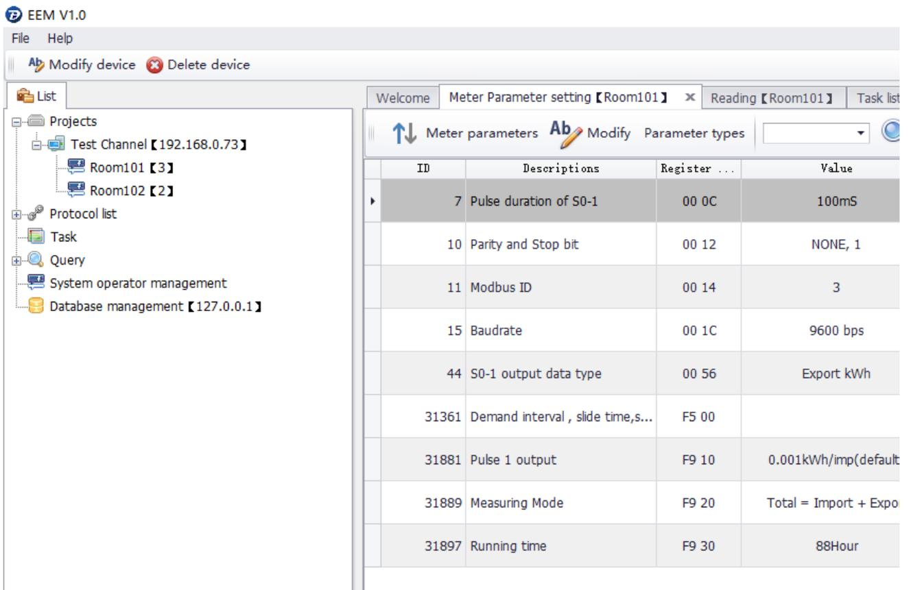
To modify a parameter, first choose the corresponding line. Then click the “Modify” button on the toolbar or the “Modify” at the end of the line. A small popup window will come out.
