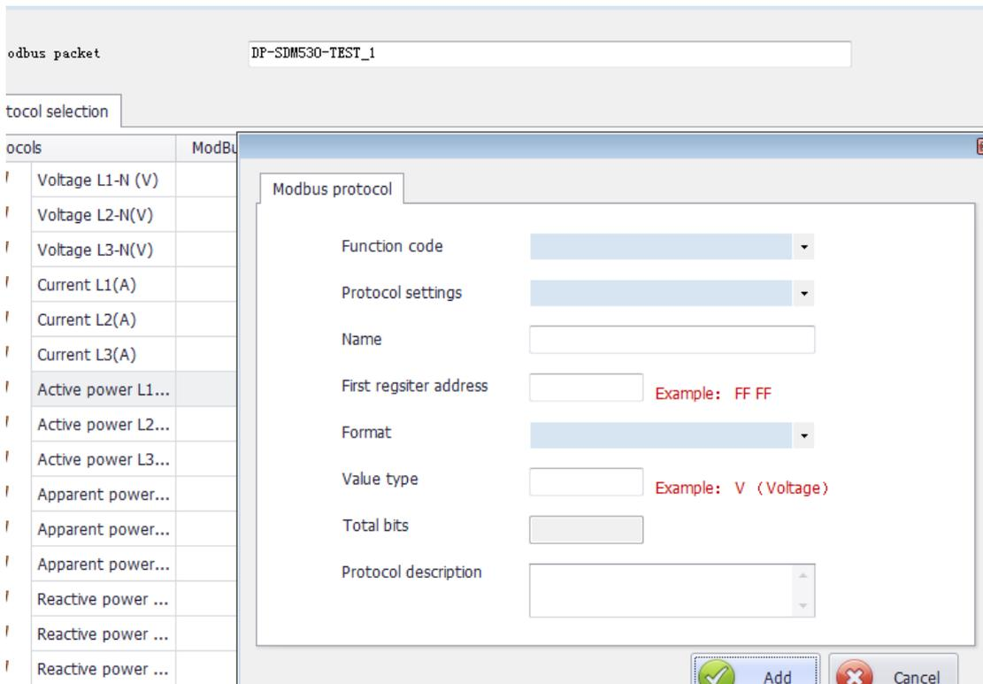
Enter parameters, press" Add", the register address also should be continuous.
