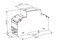
Height 99mm Width 36mm Depth 63mm
